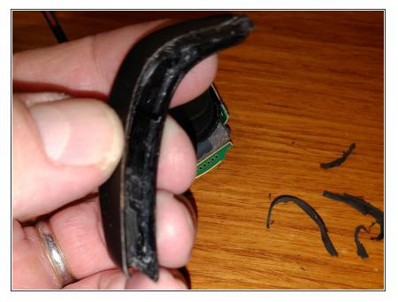
rotate the back away from the case. its basically glued in place with no other fasteners
