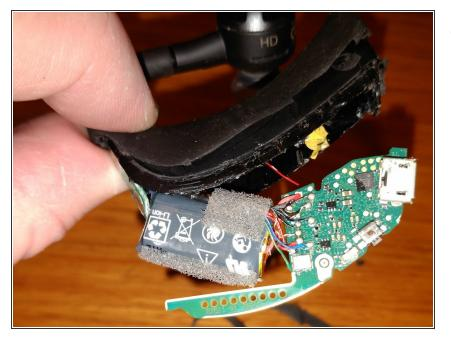
you will need to slowly cut through the foam to separate the wires from the battery. then use a soldering iron to desolder the old battery from the board these connections go through the entire board.
