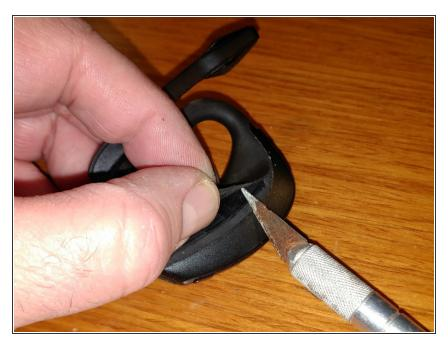
separate rubber case from back of earpiece. you don't need to remove it completely like I did.
