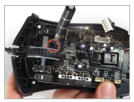
Use a Phillips #000 screwdriver to remove one 5.0 mm screw.
