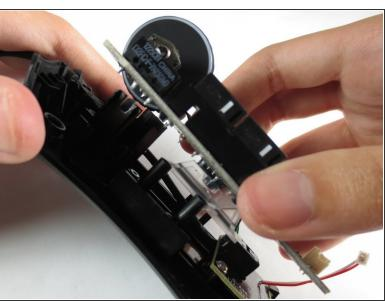
Remove the motherboard by grasping the sides and gently pulling upward.
