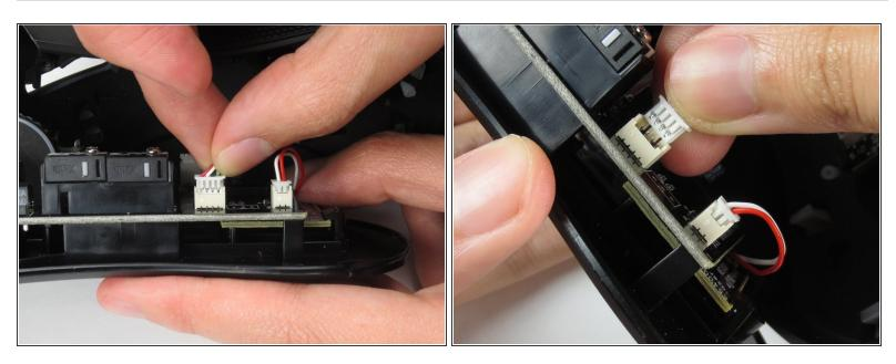
Disconnect the ribbon connector between the motherboard and the LED lights by pulling upward.
