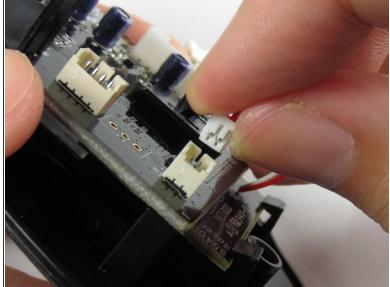
Disconnect the ribbon connector between the motherboard and the optical sensor.
