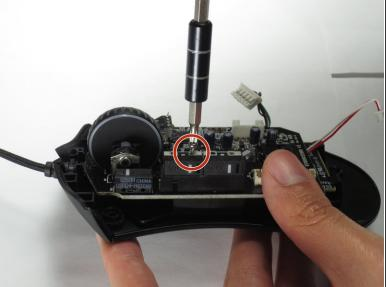
Use a Phillips #0 screwdriver to remove two 11.5 mm screws on the side buttons.
