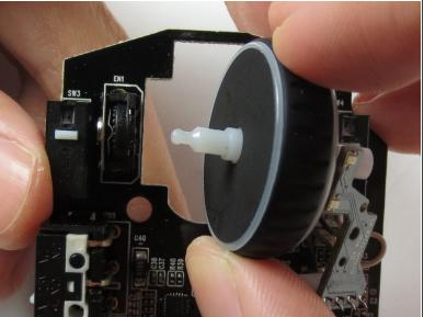
Remove the scroll wheel from the socket by pulling to the right.
