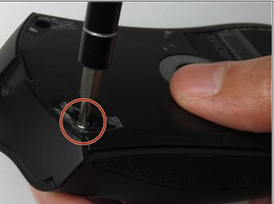
Use a Phillips #0 screwdriver to remove two 6.7 mm screws.
