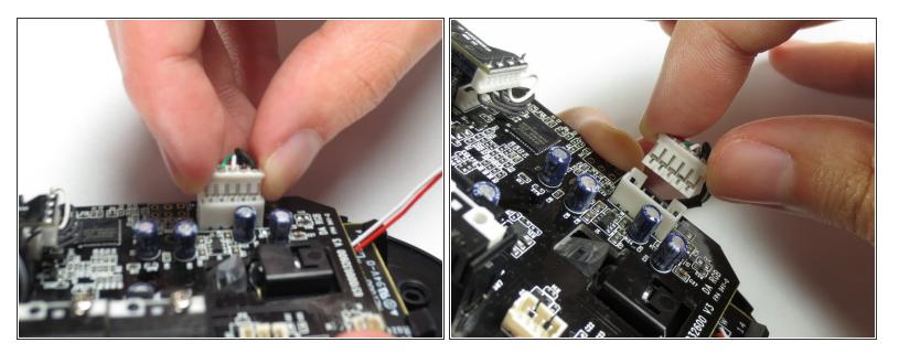
• Disconnect the ribbon connector between the motherboard and the USB cable by pulling upward.
