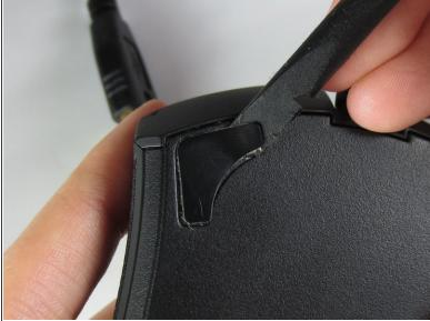
• Use the blunt end of the spudger to pry the adhesive rubber pads from the top left and right edges.
