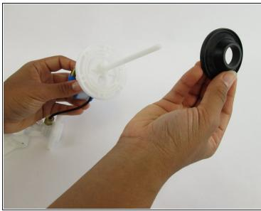
• Remove the rubber seal from the nozzle piece and replace with the new seal.
