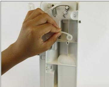
• Unhook the bottom piece of the plastic arm on each side of the device.
