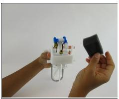
• Pull the foam pad up and remove it from the front side of the carbonation component.
