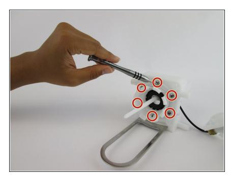
Remove the six 17.7 mm screws from the underside of the loader tab piece.
