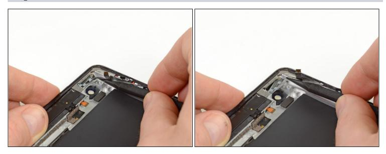
• With the tip of the spudger still underneath the ribbon cable, gently lift the power button out of its socket in the aluminum frame.
