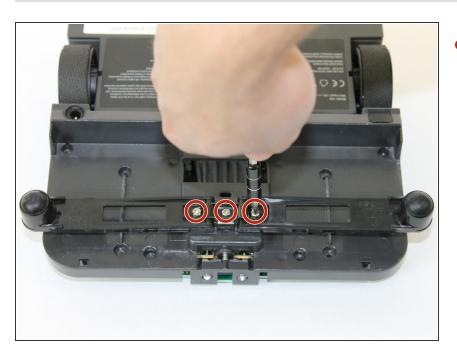
With the deck plate off, remove the three 10mm Phillips #2 screw
