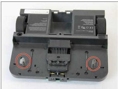
Be careful when removing the arms, do not lose the springs located under the arms.
