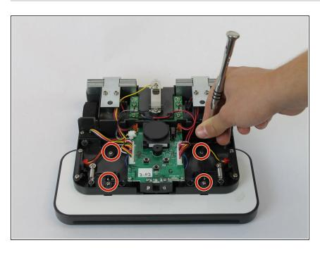
With the shell off, flip the iRobot over and remove the four 10mm Phillips #0 screws holding the deck plate assembly on.
