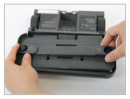
Flip the device over and remove the deck plate assembly cover by lifting it up.
