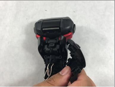
Remove the lock switch by sliding it downward until it is out of place.
