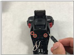
Remove the 8 mm screws directly below the lock switch.
