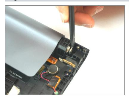
Use a spudger to pry the locking mechanism.
