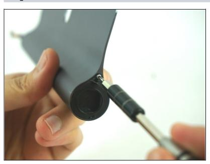
Use a small phillips-head screwdriver to remove the screw.
