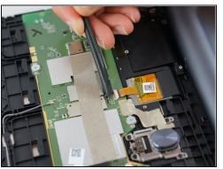
Before detaching the LCD and digitiser connectors, remove the two small screws at the top left (red bordered area in photo). Remove the metal shield and disconnect the battery wire.
