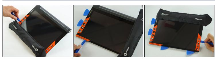
Using the plastic opening tools separate the screen from the device.
