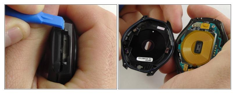
Insert a plastic opening tool between the top and bottom portions of the case, and gently pry off the back.
