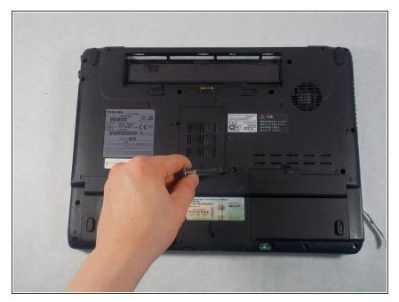
Using the #J1 bit, remove the 17 recessed 7.3 mm B6 screws from the underside of laptop and the 3.1 mm #J0 F3 screw inside the battery compartment.
