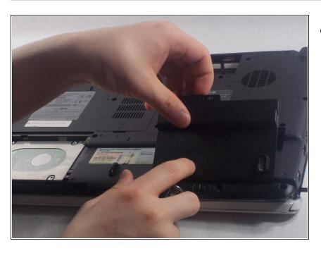
The secondary hard drive can be removed following the same process on the right drive bay.
