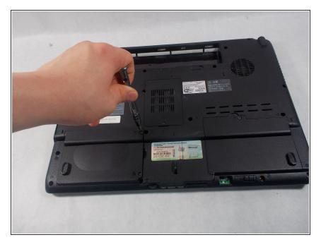
Start by using the #J1 screw bit to unscrew the the two 4.6 mm hard drive bay screws located on the underside of the laptop. They are located next to the Windows license sticker.
