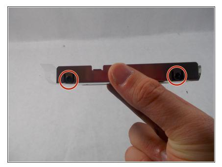
The drive can now be removed from the metal drive retainer by unscrewing the four exposed 4.1 mm #J1 screws on either side of the drive.
