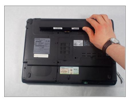
The battery is now easily removed by pulling up from the notched tab on the inside edge.
