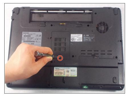
Remove the 4.5 mm screw labeled 4 and lift up panel from the vented 2" x "4 memory cover in the middle of the computer.
