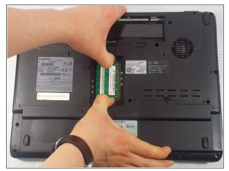
Gently pull apart the two metal support clips on either side of the chip to release from the socket. It will spring upwards when it is properly released.
