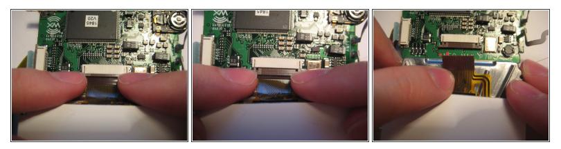
• To remove the ribbon cable from the board, catch the sides of the connector with fingernails and pull downward.
