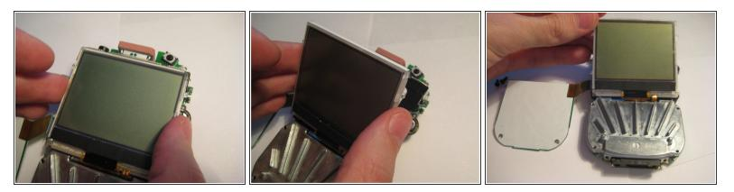
• Pivot the LCD screen, pulling on the top and sides and keeping the bottom attached.
