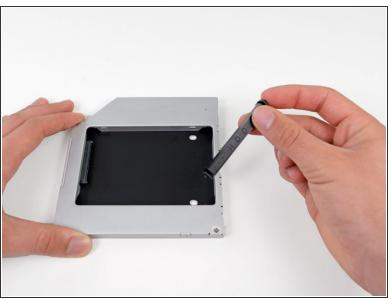
Remove the plastic positioner from the optical bay hard drive enclosure by pressing in on one of the clips on either side and lifting it up and out of the enclosure.
