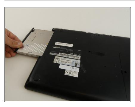
Slide out the optical drive to remove it.
