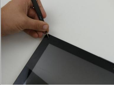
Remove the 4 rubber stoppers with the precision tweezers.
