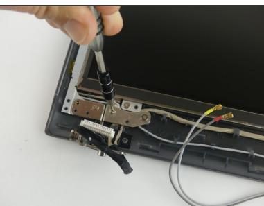
Remove the three 4 mm screws on each hinge with a Phillips #000 screwdriver. There should be a total of 6 screws to remove.
