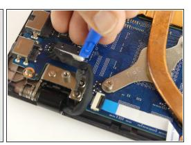
• Disconnect the wire by carefully using the plastic opening tool to pry the connector away from the motherboard.
