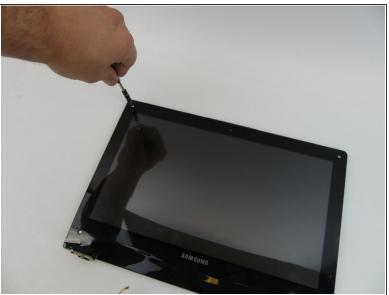
Remove the four 4 mm screws with a Phillips #000 screwdriver.
