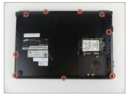
Unscrew nine 6 mm screws on the cover using a Phillips #000 screwdriver.
