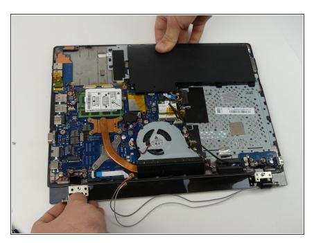
Hold hinges in place with your thumb and slide the laptop away from the screen.
