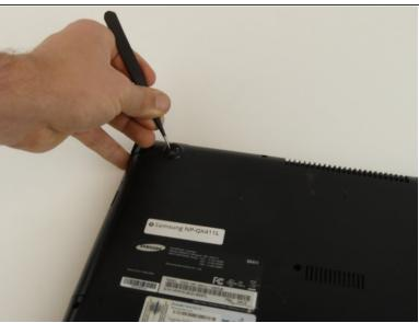
Remove the top two rubber stoppers using precision tweezers.
