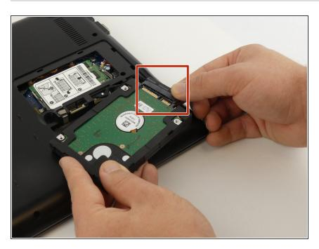
Remove the hard drive by gently pulling the power connector at the base of the wire off. You can do this by pulling the connector away from the hard drive.
