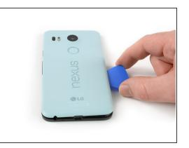
Continue to slide the opening pick around all sides of the phone to release all clips that secure the rear panel.
