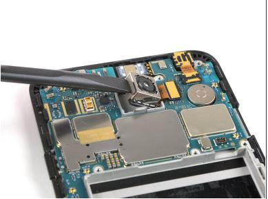
Apply the flat end of a spudger to the left side of the rear facing camera and carefully lever it up.
