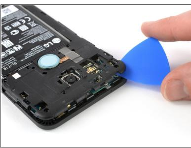
Continue sliding the opening pick around the upper part of the midframe to release the plastic clips.
