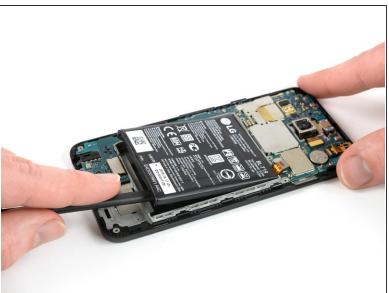
Insert the flat end of a spudger under the bottom right corner of the battery and gently pry upwards to loosen the remaining adhesive.
