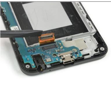
Use the flat end of a spudger to pry up the display flex connector.
