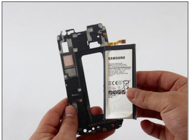
• Remove the battery from the frame.
