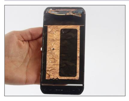
Remove the display assembly (LCD and Digitizer).
