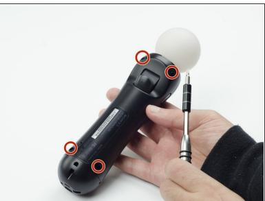
Turn the controller over and unscrew the four 10mm screws with a PH #00 screwdriver.
