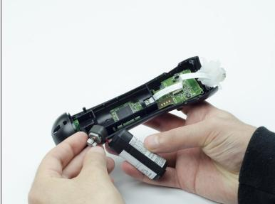
Using a plastic opening tool, carefully pry the rumble motor free.
