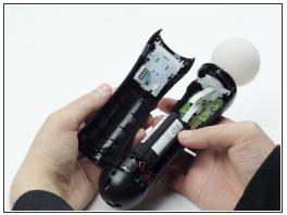
• Pinch the sides of the back panel to remove it and set it aside.
