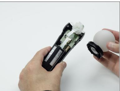
Hold the base of the controller with one hand and with the other carefully pull up on the white spherical piece to remove it.
