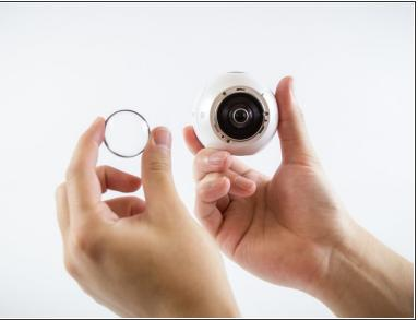
Insert flathead screwdriver into marked slot on camera lens and pry off the camera lens cover.
