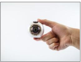
Twist silver ring on lens counter clockwise with force to remove the cover
