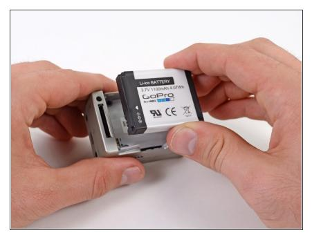
Remove the battery from the case.
