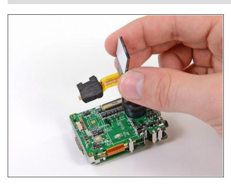
Once its ribbon cable is free, remove the LCD from the motherboard assembly. To reassemble your device, follow these instructions in reverse order.
