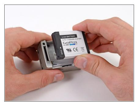
Remove the battery from the case.
