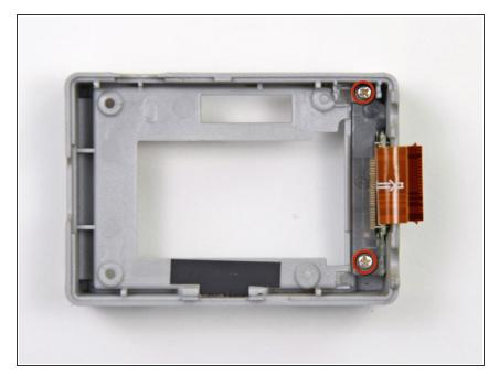
Remove the two 5.8 mm Phillips #00 screws securing the SD board cover to the rear case.
