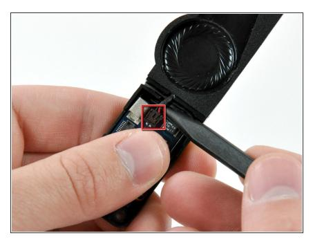
Use the pointed end of a spudger to pry the speaker connector up off the audio board.
