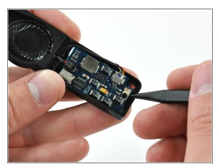
Insert the pointed end of a spudger into the gap around the audio board to pry it up off the adhesive securing it to the speaker housing.
