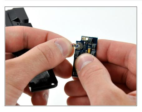
Disconnect the audio out cable by pulling its connector straight away from the socket on the audio board.
