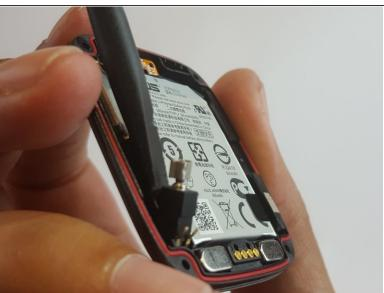
Place the spudger under the vibration motor and lift up to remove it from the watch.
