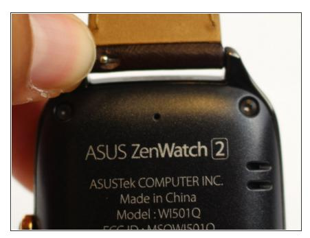
Remove the watch strap by sliding the knob inward to detach from the face plate.
