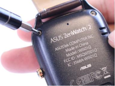
Open the watch by removing the four 3.5mm screws using the T5 screwdriver.
