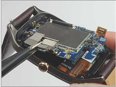
Pull up on the motherboard using tweezers to detach it from the watch.
