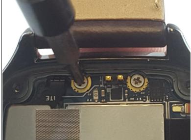
Remove the two 1.8mm silver screws using the PH00 screwdriver.
