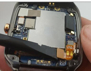
Slide the spudger under the gold-plated connection ribbon and lift to disconnect from the motherboard.
