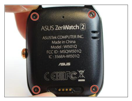
Remove the four 3.5mm screws using a T5 screwdriver to open the faceplate.
