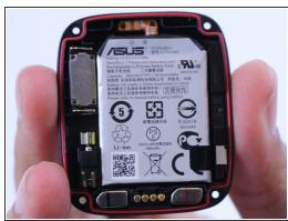
Remove the four 3.5mm screws to detach the case using the T5 screwdriver.
