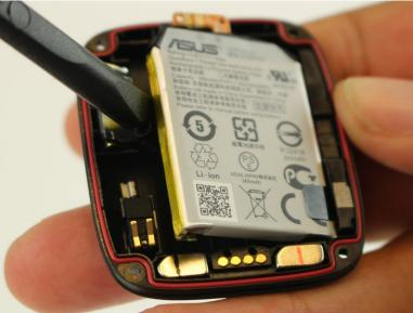
• Slide the spudger under the battery and lift to remove.
