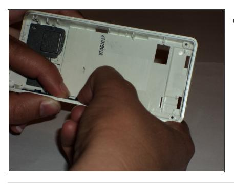
Push down on the volume button to snap it back into the case.
