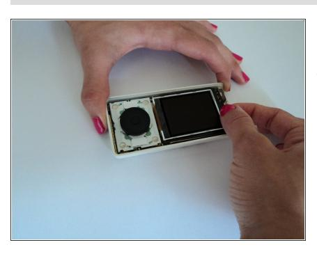
While looking down at the device, place your index finger at the top of the circuit board and your thumb on the device screen.
