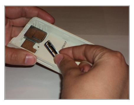
Remove the volume button from the device.
