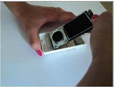
Using your fingers, gently pull the top of the circuit board up toward you while also sliding the bottom of the circuit board away from the bottom of the Sirius Stiletto 100 back cover.
