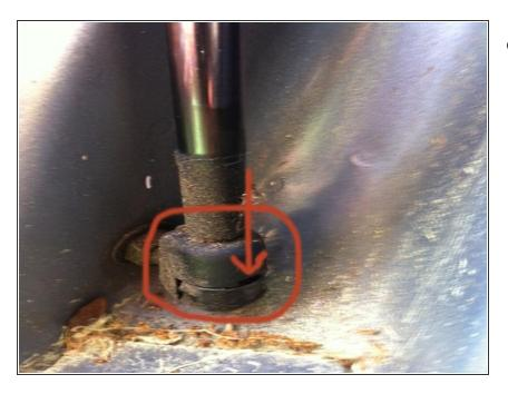
Repeat for the bottom strut. Open clip and remove strut.
