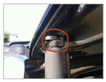
Once the clip is open, simply pull the strut away from trunk. It might require a little force, but should easily come off. You may have to lift the trunk a little.
