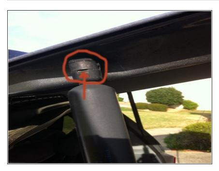
Use a small flat head screwdriver to pry open the clip. Insert the screwdriver head into the smal opening. (this picture shows the clip closed)
