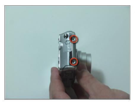
• Remove the 2 screws from the left side of the camera
