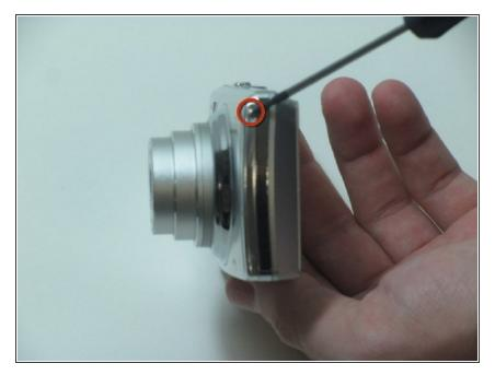
Using a Phillips head size 0 screwdriver, remove the screw from the right side of the camera
