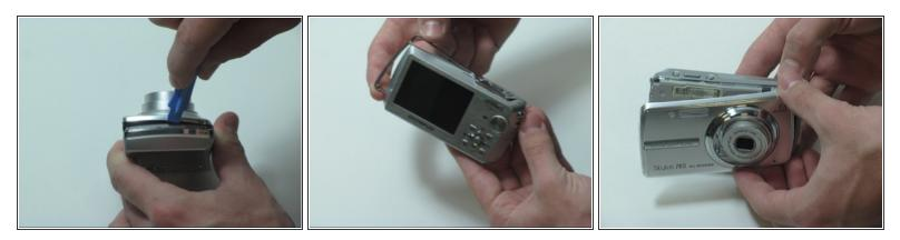
• Separate the front casing from the back using a plastic opening tool, gently.
