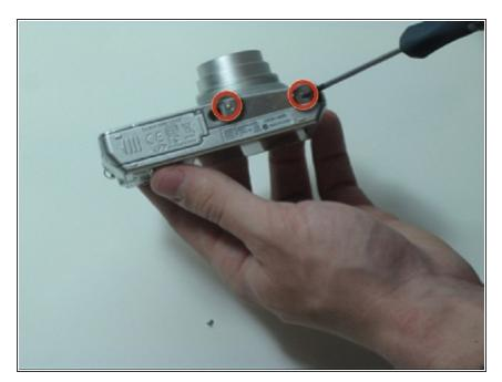
• Remove the 2 screws from the bottom of the camera
