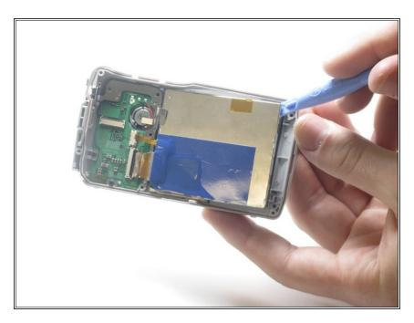
Using a plastic separating tool, remove the LCD screen from the plastic casing.
