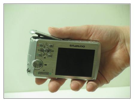
Slide the door located on the bottom of the camera in an outward direction
