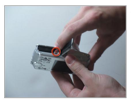
Pull back on the red release tab located on the left side of the battery.
