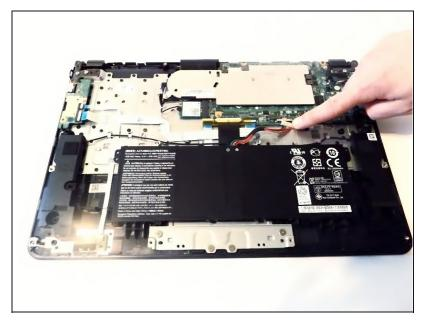
Once it is opened up, locate the battery and the cable that is attached to it.
