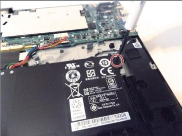
• Next, unscrew the battery pack. The one screw should be located on the far right of it. This will ensure that the battery comes out easily and affectively.
