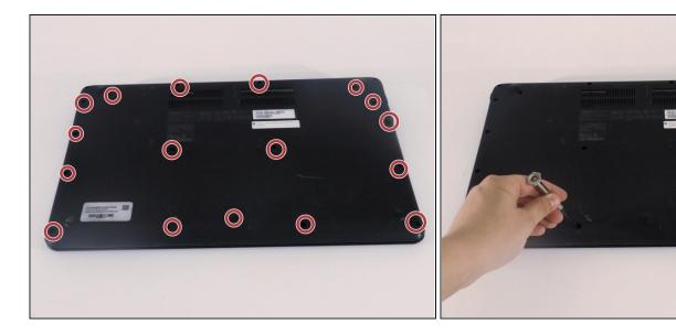
• Remove the 18 Phillips screws using a screwdriver with a PH0 bit.
