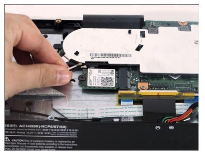
Remove the two antenna cables that attach the wireless card to the motherboard. One will be black and the other will be white.
