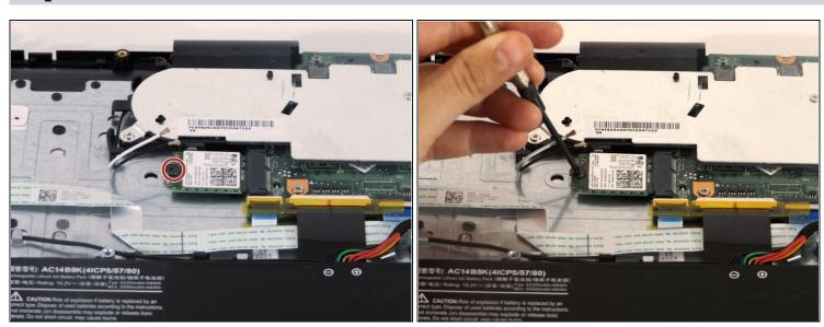
• Locate the screw that holds the wireless card in place and then remove it using a screwdriver with a PH0 bit.
