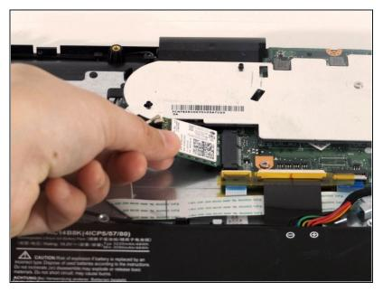
Slide the Wireless card out gently with two fingers while being careful not to damage any surrounding parts.
