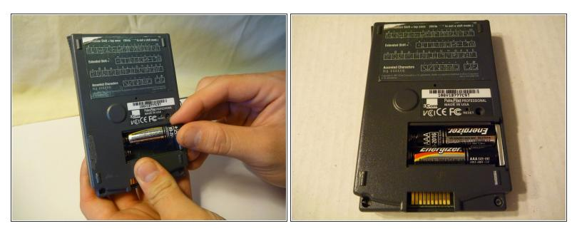
Place two AAA batteries in the battery compartment.
