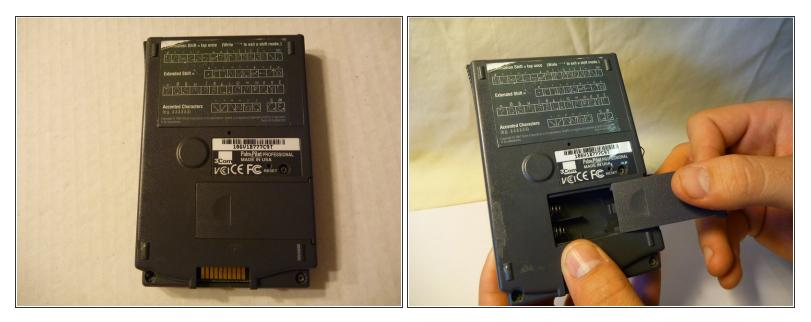
• Slide the battery cover on the back of the Palm Pilot to remove it.
