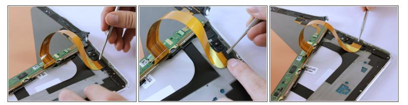
• Remove the ribbon cable using the Metal Spudger.
