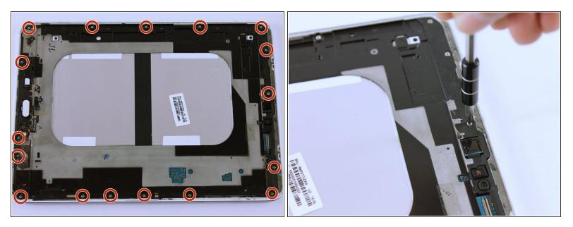
• Remove all seventeen 3 mm screws using a PH000 Phillips screwdriver.
