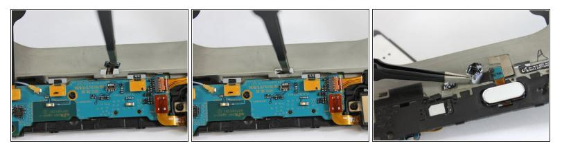
• Carefully push the cable through the hole to the other side of the frame.
