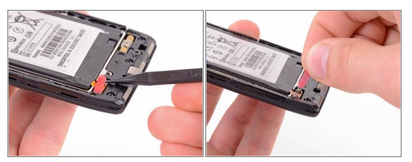
Use the tip of a spudger to lift up the red silicone cover over the battery terminal screws and remove it.
