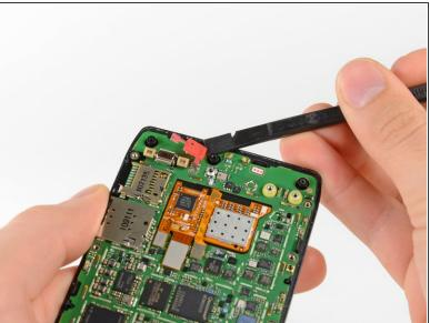
Use the flat end of a spudger to remove the two red silicone microphone covers at the top and bottom of the motherboard.
