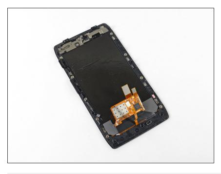
Once separated from the motherboard assembly, the entire display assembly can be replaced.
