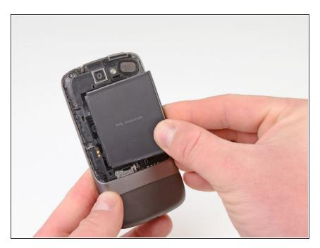
• Pull the battery up and out.
