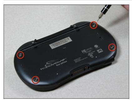
• Remove the four Torx T5 screws from the back panel.
