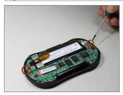
Unscrew the 2 Philips #00 screws on each end of the motherboard.
