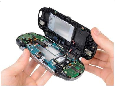
Gently separate the two cases, minding the battery and the touch screen controller connectors holding the two cases together.
