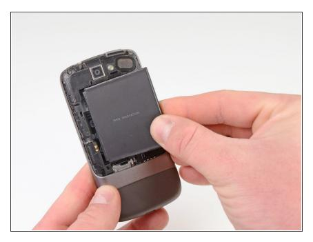
Pull the battery up and out.
