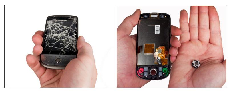
• Tilt the inside of the front enclosure towards your cupped palm to remove the trackball and it's enclosure will fall out.
