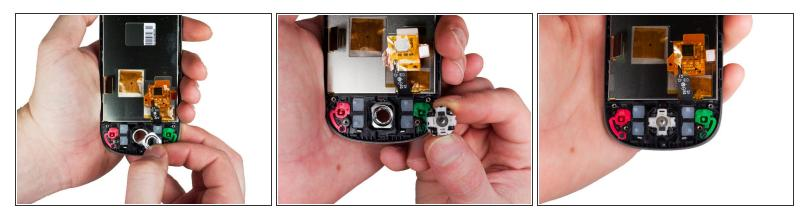
• Position the phone off of the edge of the table and insert the replacement part by inserting the bevel then the trackball into the hole.
