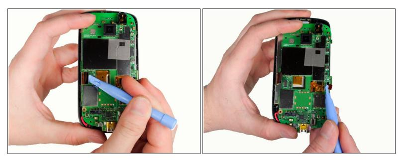
• **Gently** pull off the ribbons holding the sides of the motherboard to the front enclosure.
