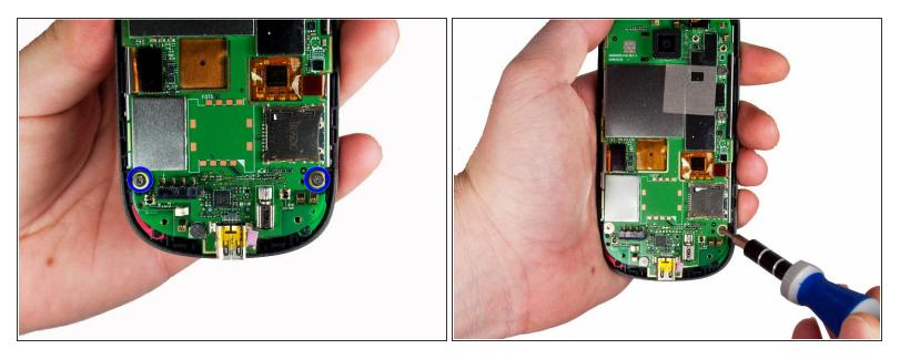
• Remove the two screws near the bottom of the motherboard with a Phillips head screwdriver.
