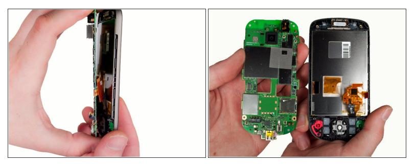
• Remove the motherboard from within the front enclosure.
