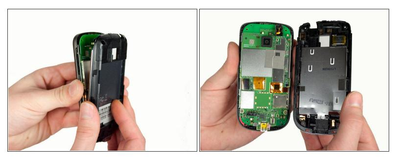
• **Carefully** separate the front and back enclosures once all of the clips have been disengaged.
