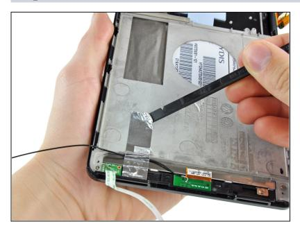
• Use the flat end of a spudger to peel up the silver tape securing the antenna cable.
