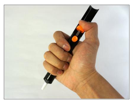
Trigger the desoldering pump before heating the solder.
