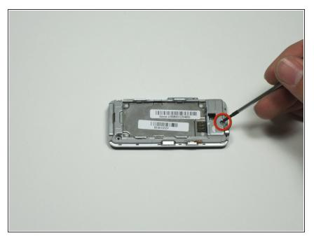
Remove the single 0.327" silver screw on the back of the device that was exposed when you removed the rear case cover.
