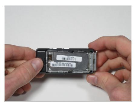
Slide the rear case cover toward the top of the device with your thumb to release it.
