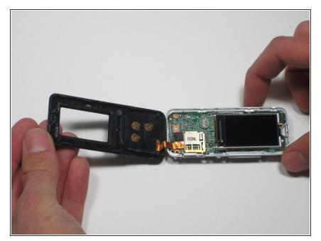
• Open the case cover starting on the side most distance from the buttons.
