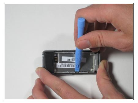
Using a plastic opening tool, pry up the two arms of the case cover near the middle of the device to free them from the sides.
