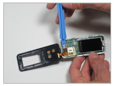
Using a plastic opening tool, gently pry up on the top of where the ribbon cable attaches to the motherboard to release the cable.
