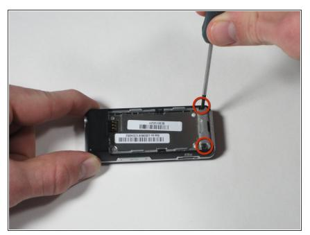
• Remove the two black .265" screws at the base of the device.
