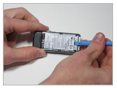
Apply a fingernail or a plastic opening tool to the base of the battery.
