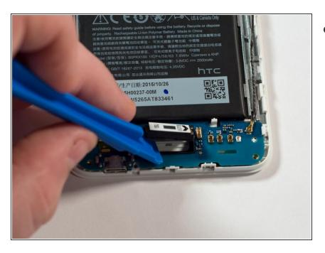
Place the plastic opening tool under the speaker and pry it away from the device.
