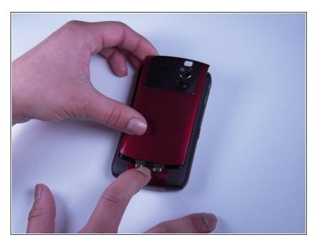
Press down on the battery release button and slide the back cover up with your thumb.
