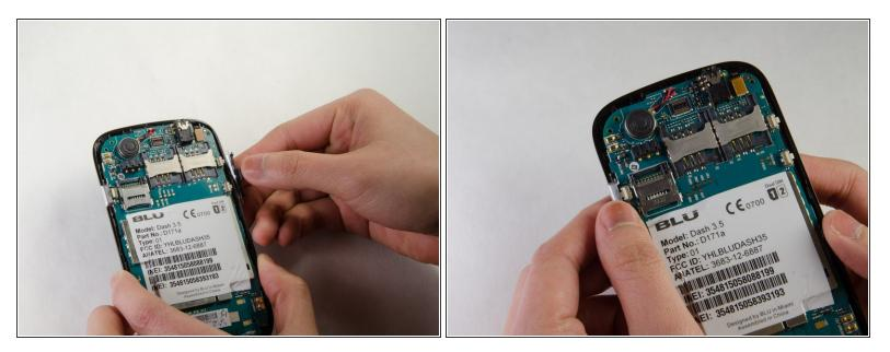
• Remove volume and lock buttons by lifting them gently from the casing.
