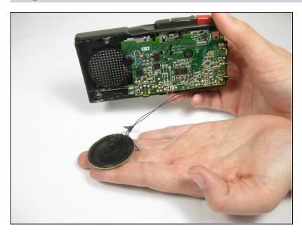
Now that the speaker is detached from the device, simply tilt the device over and let the speaker fall out. To reassemble your device, follow these instructions in reverse order.
