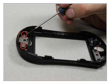
Unscrew the 2 silver Philips #00 screws from both sides of the directional pad component on the front casing.
