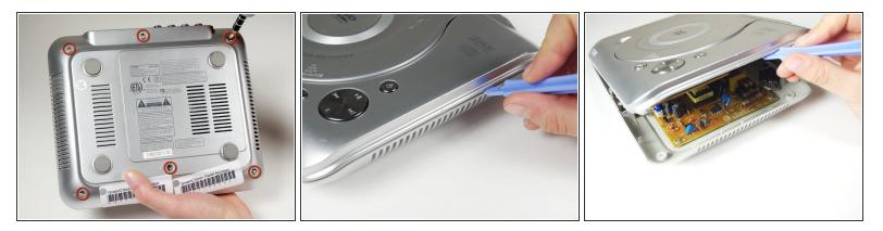
• Remove the six 1cm screws on the bottom of the device with the Phillips #1 screwdriver.
