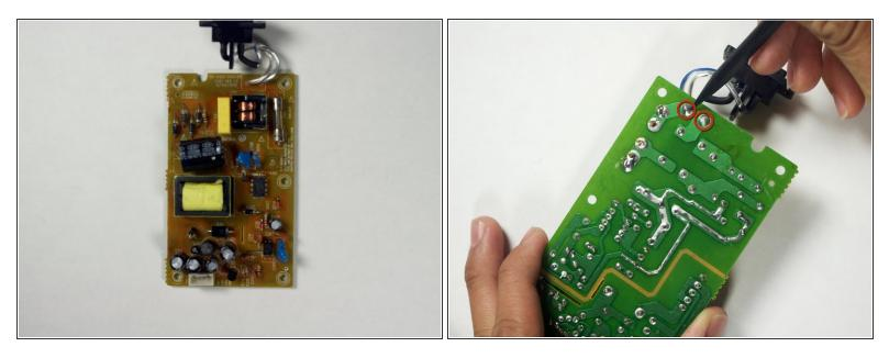
On the circuit board with the Power Port, de-solder the circled areas on the back to remove the Power port.
