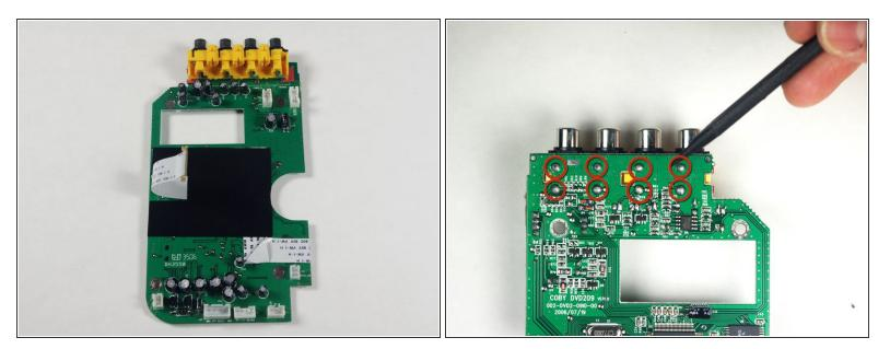
On the circuit board with the AVI Port, de-solder the circled areas on the back to remove the AVI Port.
