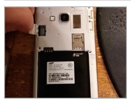
Remove the battery, SIM card, and memory card.
