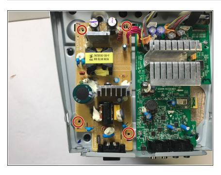
Remove the four 6.4mm phillips head screws located at each corner of the daughterboard with a Phillips head screwdriver.
