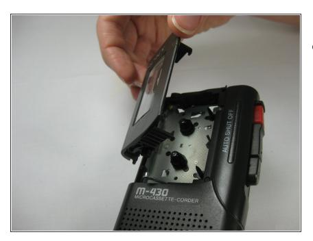
Carefully lift the cassette lid, making sure the tab and latch are free from connection.
